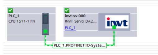
After correct configuration, add the library function SinaParaS to the program block, set and define the variables of the function block, download the project to the PLC, run the PLC, and set the project to online.
