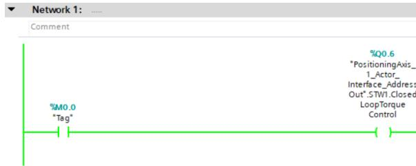
**Note:** When the torque switchover is performed through the control word STW1.14, the servo must be disabled through MC\_Power before switching from torque mode to position mode; otherwise, the servo will run at the maximum speed to the position before the switchover.
