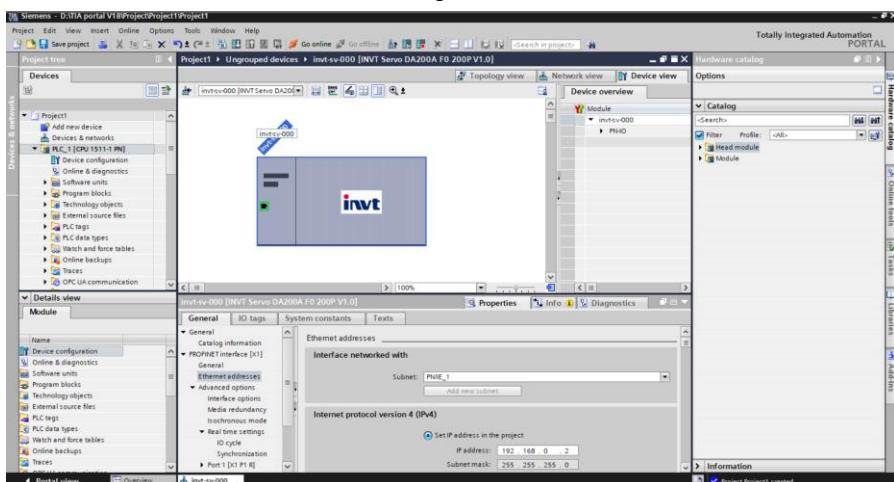
Step 5 Choose the **INVT Servo DA200A F0** device. In the **Properties** panel, click the **General** tab, and choose **PROFINET interface [X1] > Ethernet addresses**. In this tab, you can modify the default assigned IP address of the INVT Servo DA200A device.
