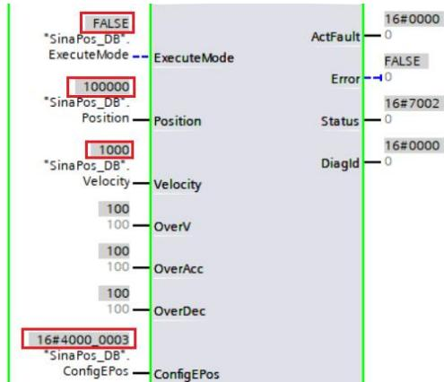
The axis starts from the initial position and approaches the target position at a set speed. The fixed stop point must be between the initial position and the target position. The set torque limit takes effect from the beginning and the Err22-0 position overrun fault is invalid when the Run to fixed stop point function is activated.
