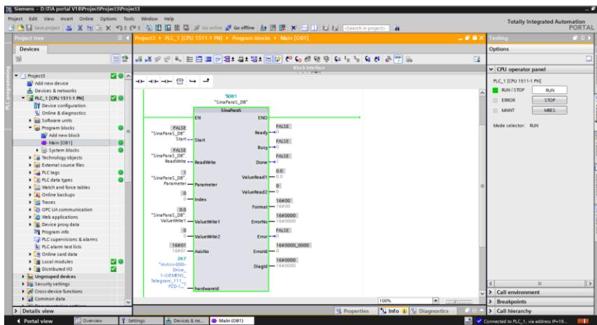
**Note:** For the DA200A-F servo drive, the default value of AxisNo in SinaParaS is set to 1.
