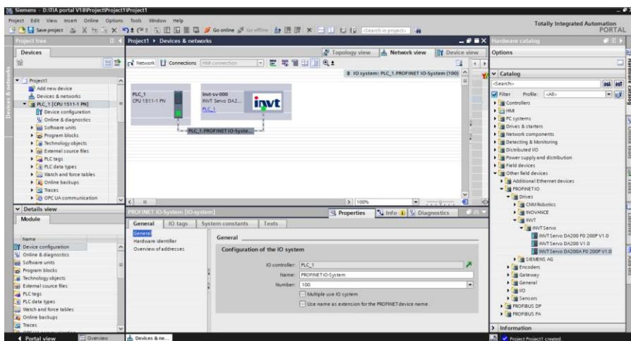
Step 4 Double-click the **INVT Servo DA200A** icon to enter the device view. Click the **INVT Servo DA200A F0** device to change its default device name.
