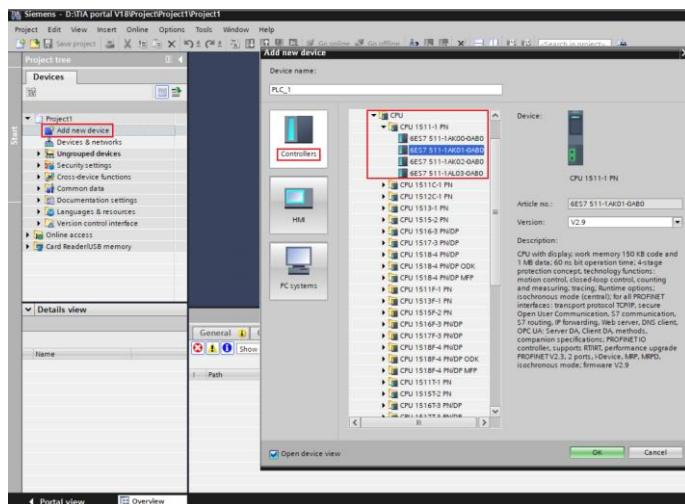
Step 2 Click **OK** and open the device view. You can select the PLC device to modify its default device name.
