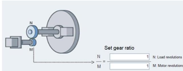
The modal axis function resets the position signal to zero after traveling a defined distance. When applied to a rotary axis, the angular position will reset to zero after a certain angle of rotation. When applied to a linear axis, the position signal will reset to zero after moving a certain distance.
