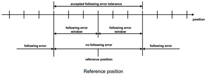
Step 3 Set P3.50 (IND = 1700) to adjust the positioning completion range (unit: user unit).
