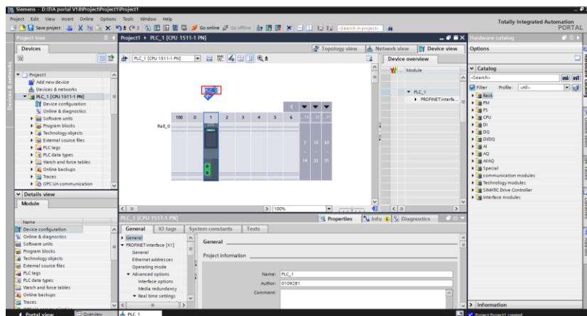
Step 3 Choose the PLC device. In the **Properties** panel, click the **General** tab, and choose **Ethernet addresses**. In this tab, you can modify the default assigned IP address of the PLC.
