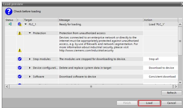
Step 5 Transfer the project to online. Speed axis control is available through the MC motion control function block.
