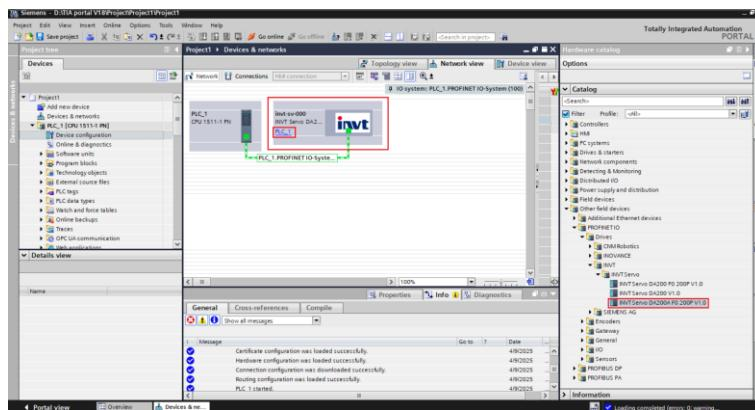
The GSD file for the DA200A-F can be installed by choosing **Options > Manage general station description files (GSD)** from the top menu bar.
