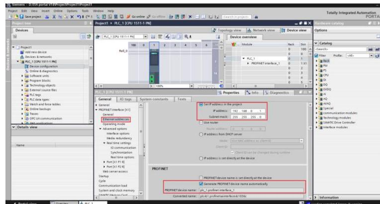
(2) Set the IP address and device name for DA200A-F.
