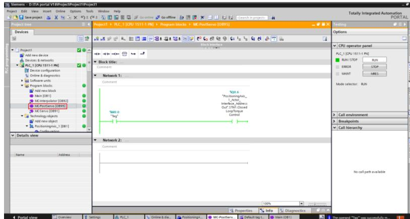
**Note:** When the torque switchover is performed through the control word STW1.14, the servo must be disabled through MC\_Power before switching from torque mode to position mode; otherwise, the servo will run at the maximum speed to the position before the switchover.
