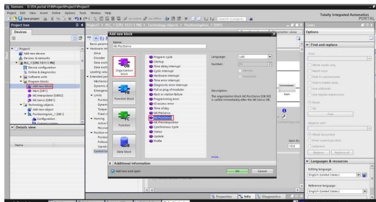
Program the MC\_PostServo function block to perform the closed-loop torque control switchover for SIEMENS telegram 102 and 105.
