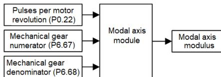
$$\text{Modal axis modulus} = \text{Number of pulses per motor revolution (P0.22)} * \frac{\text{Mechanical gear numerator (P6.67)}}{\text{Mechanical gear denominator (P6.68)}}$$
