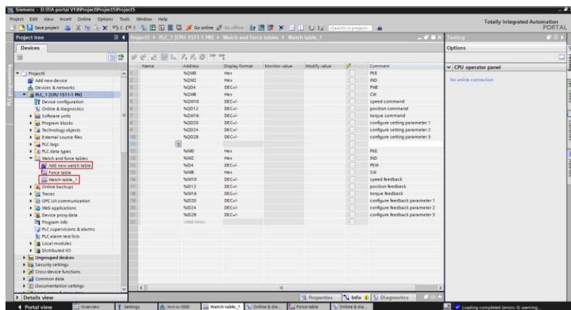
Step 2 Download the configuration and compile it to the PLC, and then enter online simulation mode. Click on the red box icon to monitor and modify parameters
