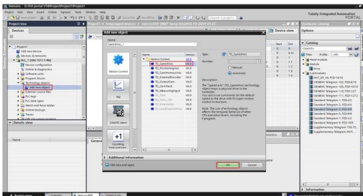
Step 2 Select the DA200A PN device Drive\_1 as the drive.
