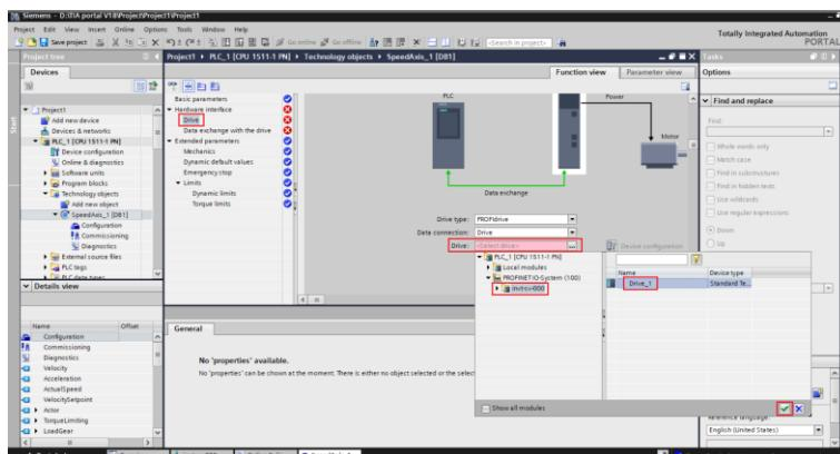
Step 3 For data exchange with the drive, do not choose **Automatically apply drive values at runtime**. Set the motor rated speed in the **Reference speed** field and the motor maximum speed in the **Maximum speed** field.
