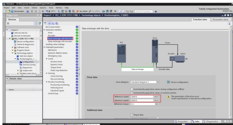
For data exchange with the encoder, do not choose **Automatic data exchange for encoder values**.
