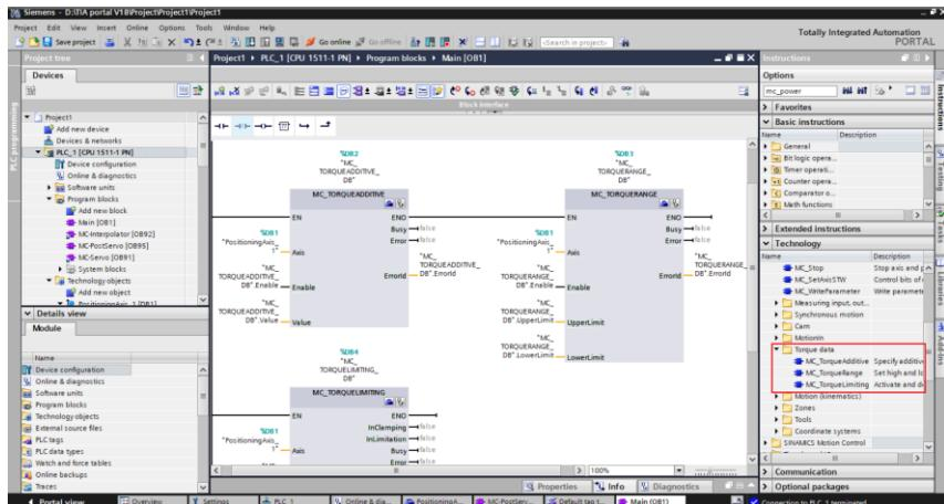
Set the control word STW1.14 to 1 through SIEMENS telegram 102/105 to switch the servo to torque control.
