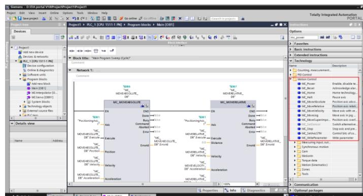
If the technology object is a positioning axis, the following MC function blocks are available: MC\_Power, MC\_Reset, MC\_Halt, MC\_MoveAbsolute, MC\_MoveRelative, MC\_Velocity, MC\_Jog, and MC\_MoveSuperimposed
