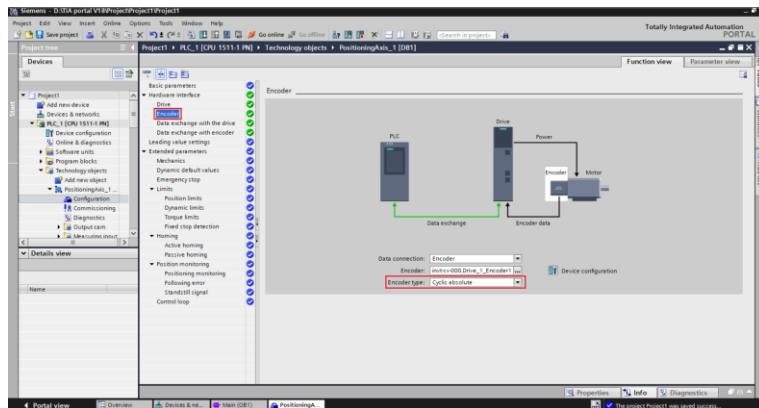
For data exchange with the drive, do not choose **Automatically apply drive values at runtime**.
