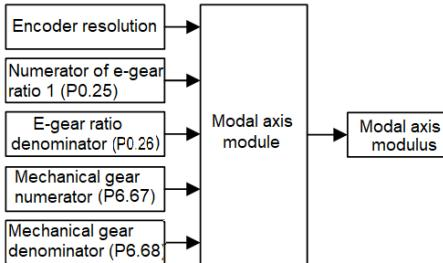
$$\text{Modal axis modulus} = \text{Encoder resolution} / \frac{\text{Numerator of e-gear ratio 1 (P0.25)} * \text{Mechanical gear numerator (P6.67)}}{\text{E-gear ratio denominator (P0.26)} * \text{Mechanical gear denominator (P6.68)}}$$
